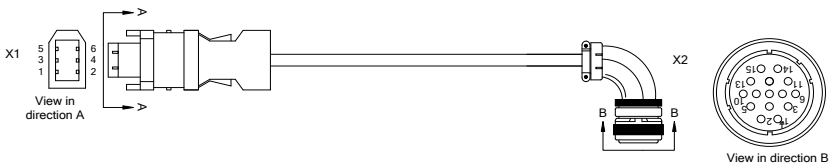
Figure 4-13 Wiring for absolute encoder of motors
